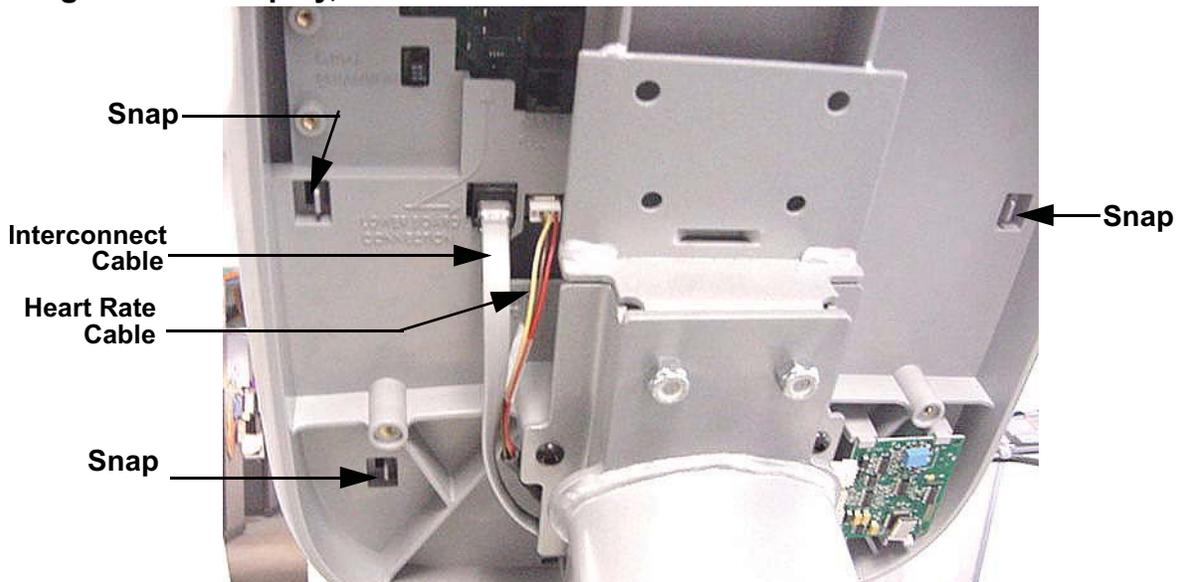
6. Starting from the top and working downward, unsnap the display front panel from the display. There are six snaps retaining the display front panel. See Diagram 7.1.
