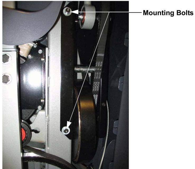
5. Set the replacement H-brake in its mounting position, If possible have an assistant support the H-brake, and replace the four H-brake mounting bolts removed in step 4. Torque the H-brake mounting bolts to 200-250 inch pounds (17 - 21 foot pounds).
