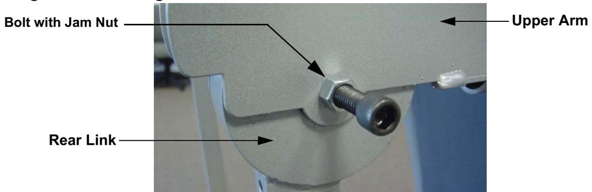
7. Separate the upper arm from the rear link. Slide the lower half of the upper cover and the lower cover off of the rear link.
