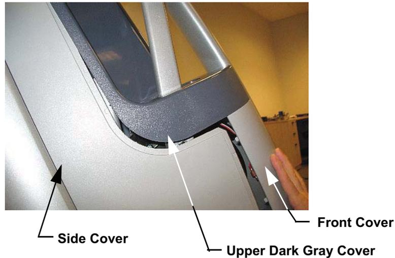
9. Set the right rear side cover in its mounting position and engage the tab at the front of the cover in the clip in the lower cover. Set the left rear side cover in its mounting position and engage the tab at the front of the cover in the clip in the lower cover. Engage the tab and clip at the rear of the left and right rear side covers. See Diagram 7.22. Fasten the left and right rear side covers with the screws removed in step 2.
