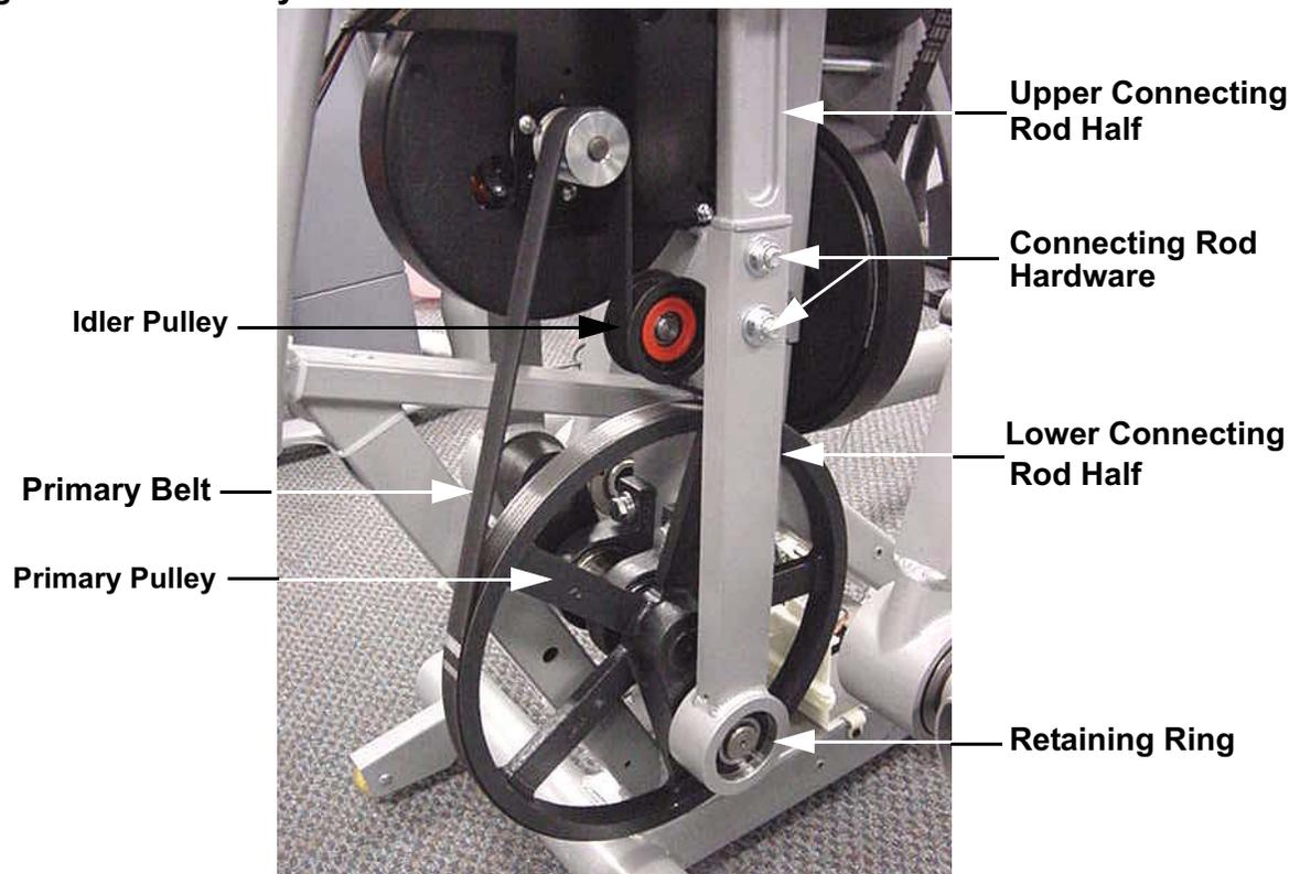
4. Remove the hardware that fastens the upper and lower connecting rod halves together. Separate the lower connecting rod half from the upper connecting rod half. See Diagram 7.4.
