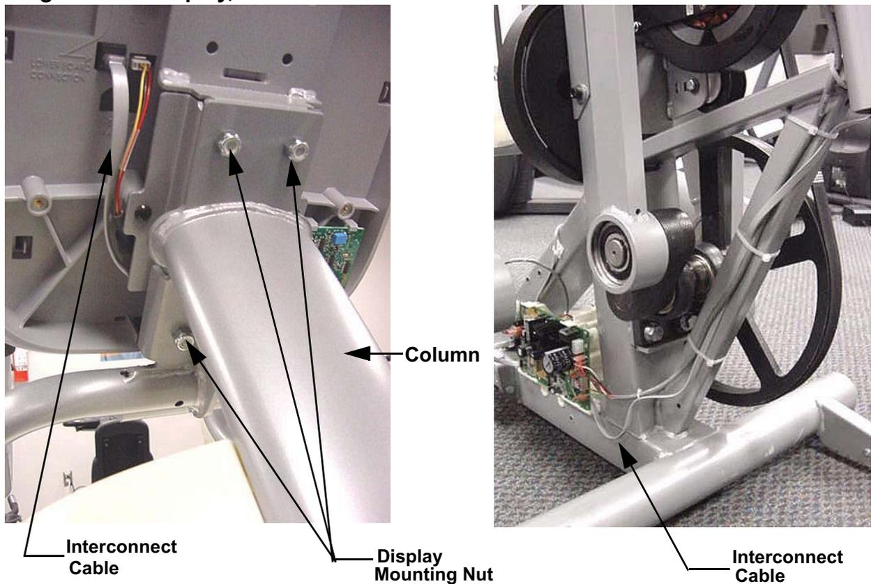
3. Remove the four nuts that fastens the display to the column. Remove the display and set it aside. See Diagram 7.3.
