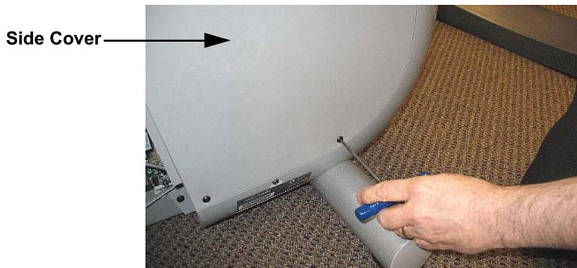
5. Remove two screws from the lower portion of the front cover. Grasp the lower portion of the front cover and remove the front cover. See Diagram 7.20.
