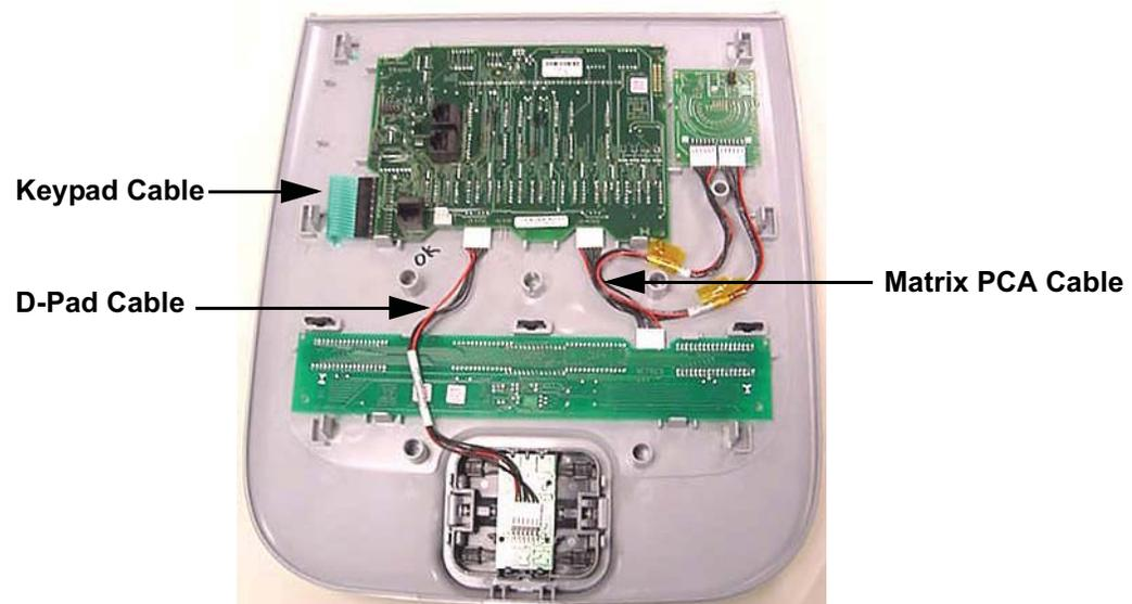
7. If a “stuck key” message is immediately displayed when the C100i is powered up, replace the upper PCA.
