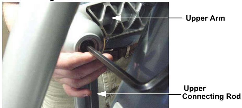
5. Remove the large end cap from the center of the upper.
