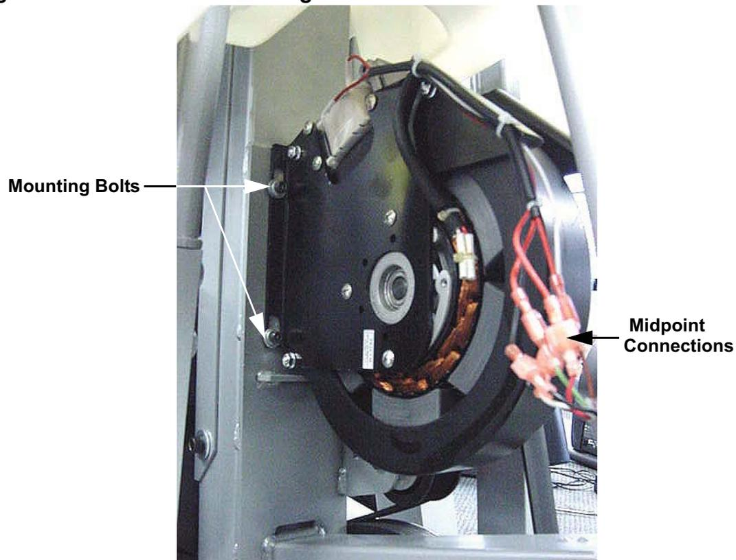
5. Remove the four generator mounting bolts and remove the generator.
