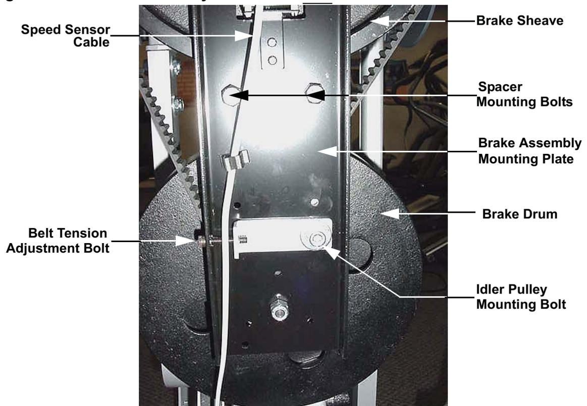
7. Remove the four screws from the belt bracket and remove the belt bracket. Remove the brake belt by lifting it over the top and bottom edges of the brake assembly mounting bracket.
