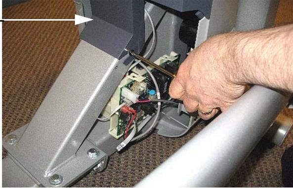
4. Remove two screws from the bottom edge of both side covers and remove both covers. See Diagram 7.19.
