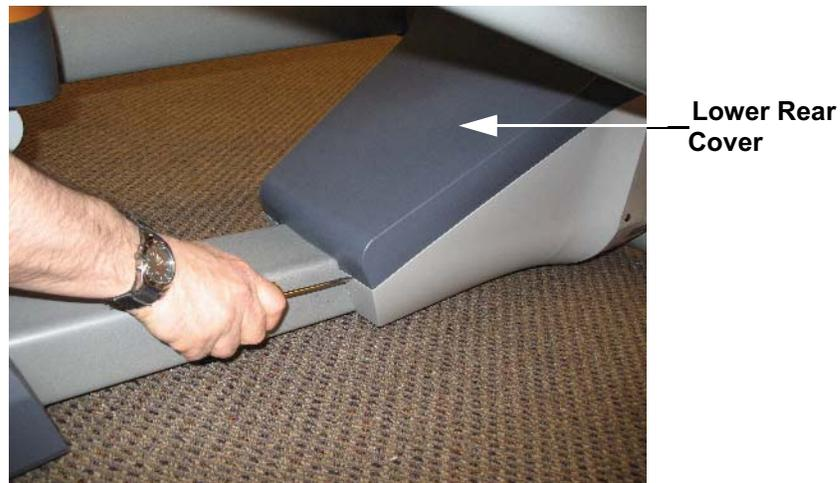
2. Remove two screws, one each side, from left and right lower rear side covers. See Diagram 7.17. Depress the tab at the rear of the covers and remove the left and right rear side covers.
