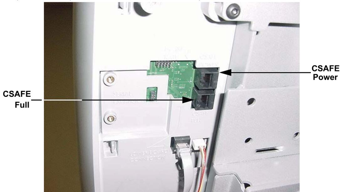
3. Connect the computer interface cable to the CSAFE Full port.
