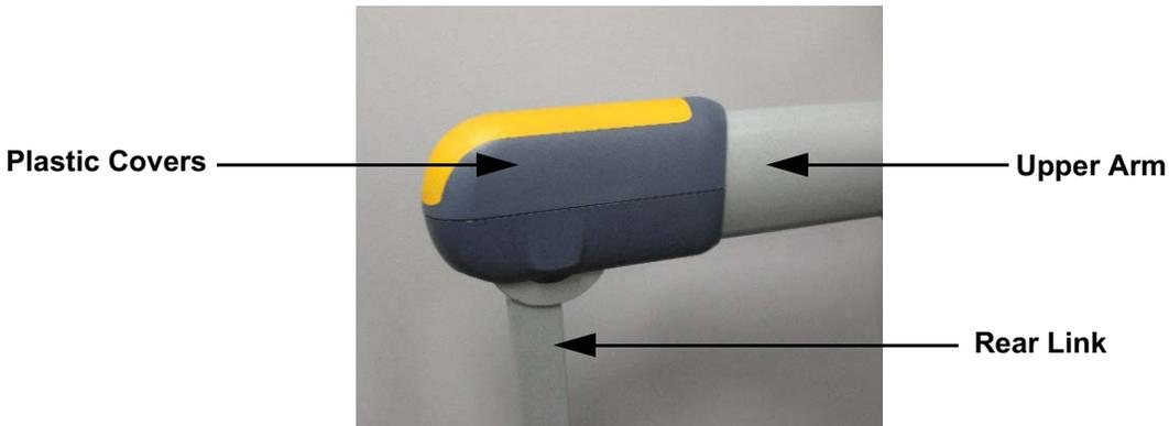
2. Place a 9/16" end wrench on each of the hex head bolts that fasten the upper arm to the rear link. These bolts thread into a free floating shaft, remove one of the two bolts.
