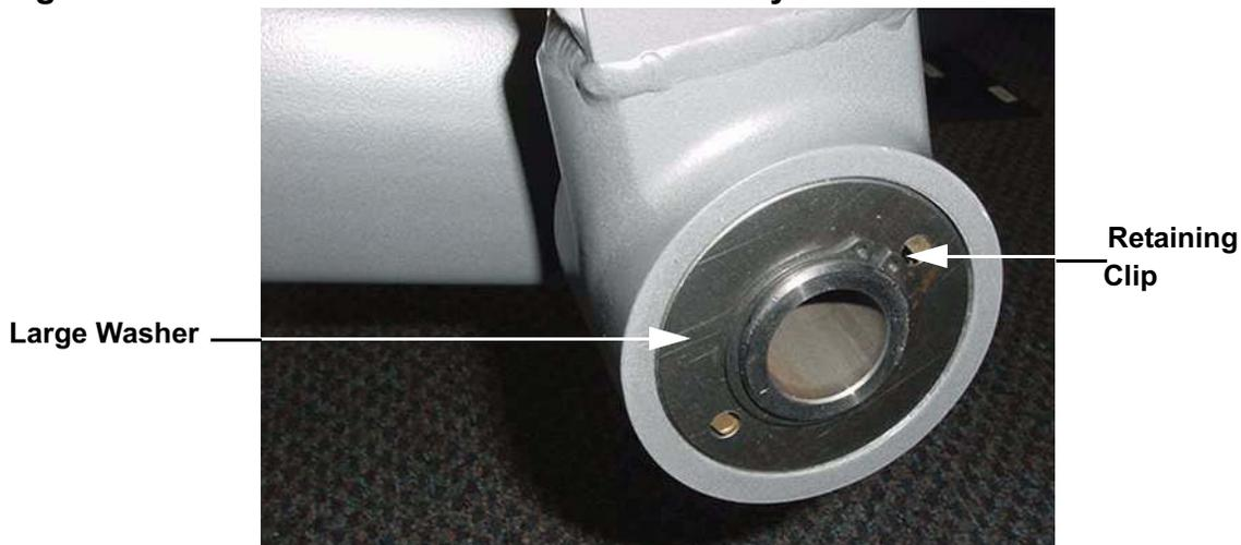
4. Remove the stairarm from the front arm assembly.
