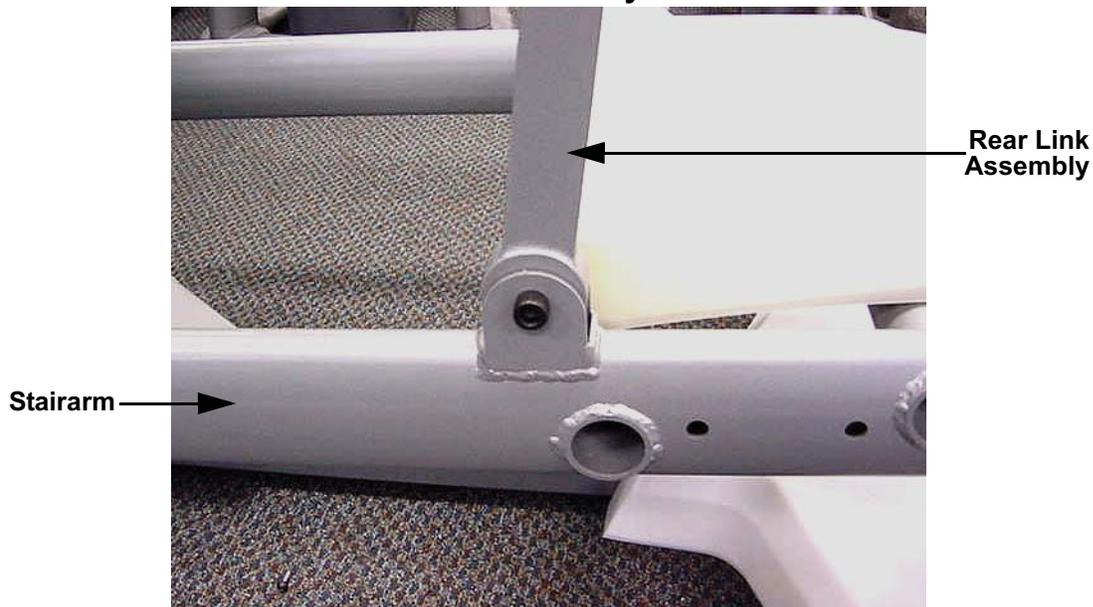
3. Remove the retaining clip and large washer that fastens the front of the stairarm to the front arm assembly. See Diagram 7.10.
