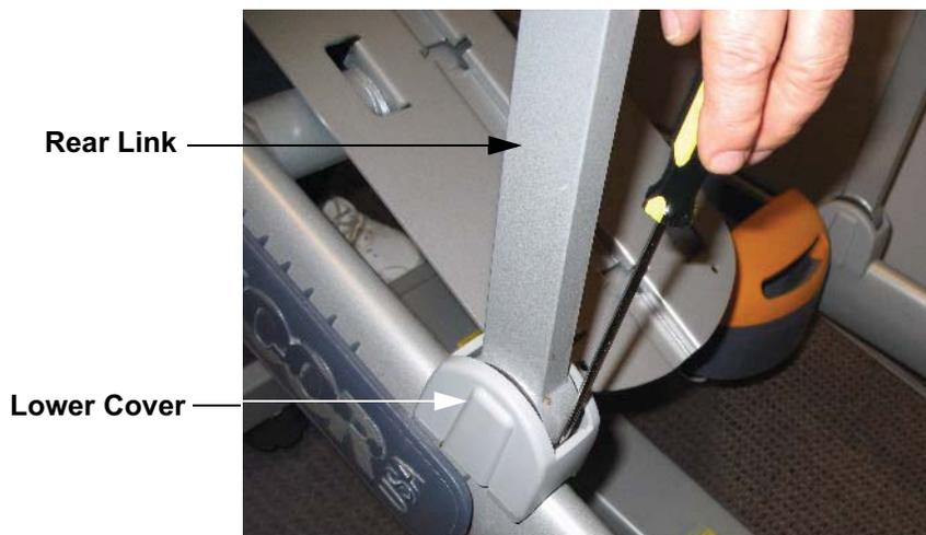
3. Place a 9/16" end wrench on each of the hex head bolts that fasten the upper arm to the rear link. These bolts thread into a free floating shaft, remove one of the two bolts.
