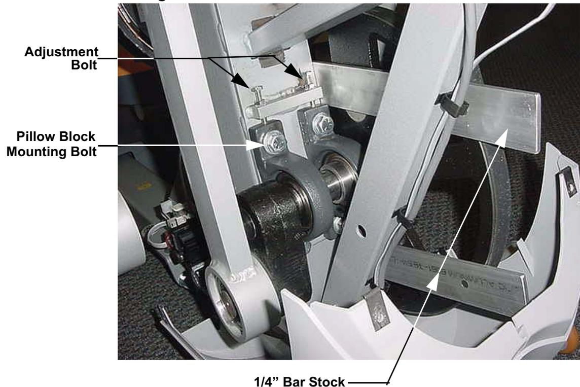
3. Slide two pieces of 1/4" inch thick bar stock between the upper and lower portions primary pulley and the frame as shown Diagram 5.4.
