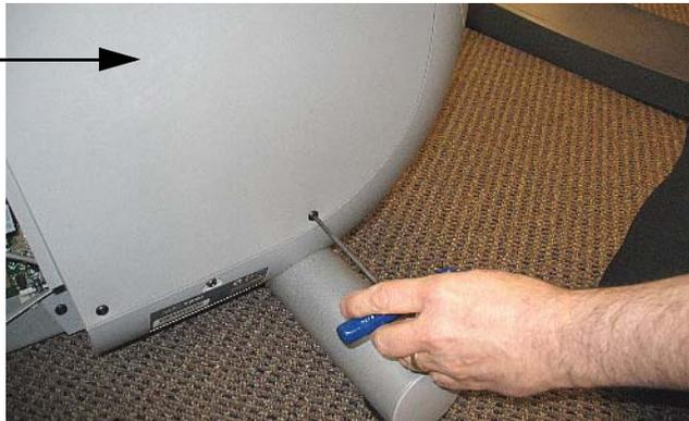
5. Remove two screws from the lower portion of the front cover. Grasp the lower portion of the front cover and remove the front cover. See Diagram 7.20.
