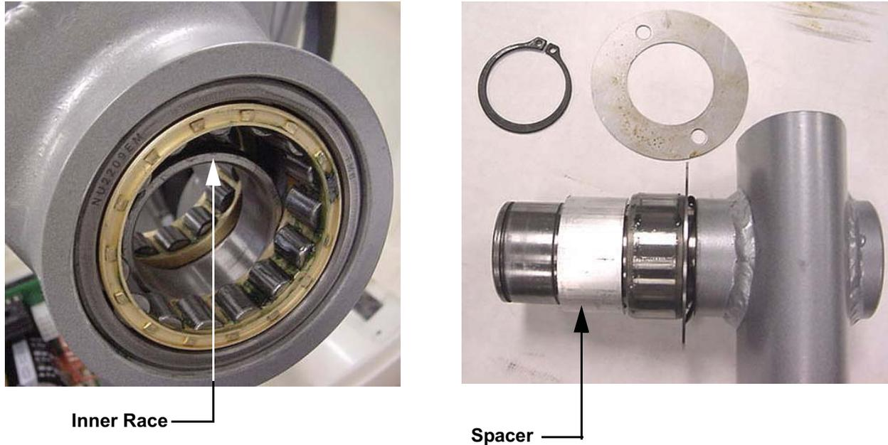
7. Left hand view of Diagram 7.11 shows that the inner race of the far bearing has fallen into the space between the bearings. This race must be slid back into the far bearing. The right hand view of Diagram 7.11 shows that the inner race of the near bearing has stayed on the stairarm. This arrangement is typically what happens when the stairarm is removed.
