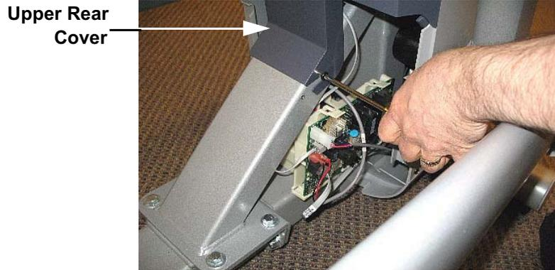
4. Remove two screws from the bottom edge of both side covers and remove both covers. See Diagram 7.19.
