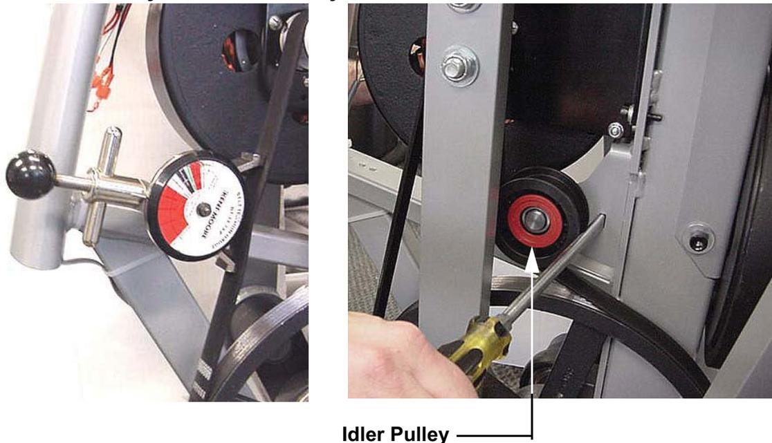
3. The belt gauge should read approximately 70 lbs. If the belt tension is significantly high or low the belt tension may be adjusted by loosening the idler pulley mounting bolt and carefully prying against the idler pulley to obtain the correct belt tension. When the belt tension is correct, torque the idler pulley mounting bolt to 17 - 21 foot pounds (200 - 250 inch pounds).
