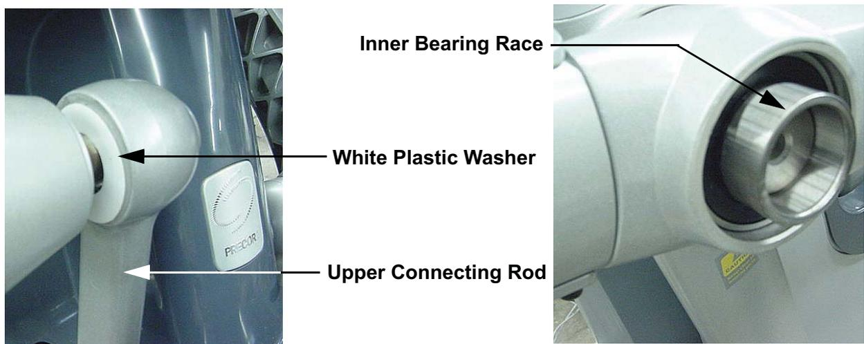
11. Slide the large black washer, removed in step 8, onto the upper arm mounting shaft and fasten the upper arm with the snap ring removed in step 8. replace the large end cap removed in step 6. It may be necessary to replace the large end cap if it no longer fits securely in the upper arm.
